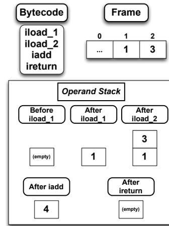
Figure 2: In this example we are assuming that the frame already contains the local variables 1 and 3 to retain simplicity. When `iload_1` is executed, it takes the element from the frame at index 1 and pushes it onto the stack. `iload_2` does the same thing but with index 2. `iadd` pops two elements from the stack, which both must be of integer type, adds them and then pushes the result to the stack. `ireturn` simply pops the stack and returns that element.
