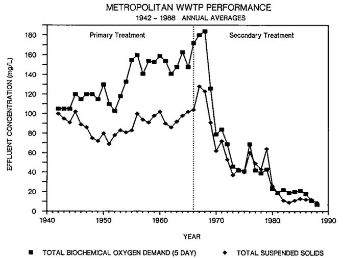
Figure 4. Metropolitan Wastewater Treatment Plant performance from 1942-1988, as measured by total biochemical oxygen demand (5-day) and total suspended solids.
