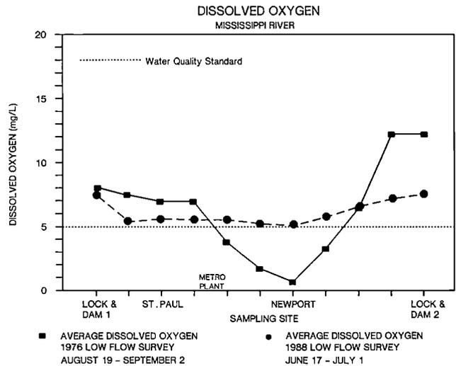
Figure 5. Dissolved oxygen concentrations in the Mississippi River, from Lock and Dam 1 to Lock and Dam 2, under low flow conditions: 1976 and 1988.
