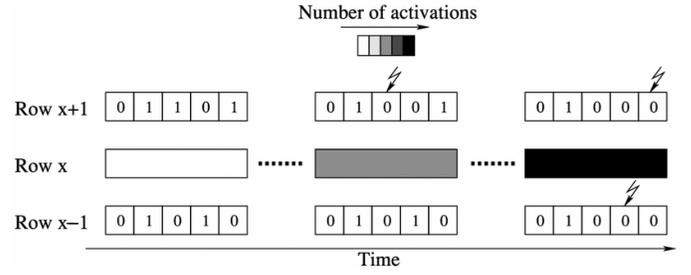
**Figure 2: Double-sided hammering** [6].
