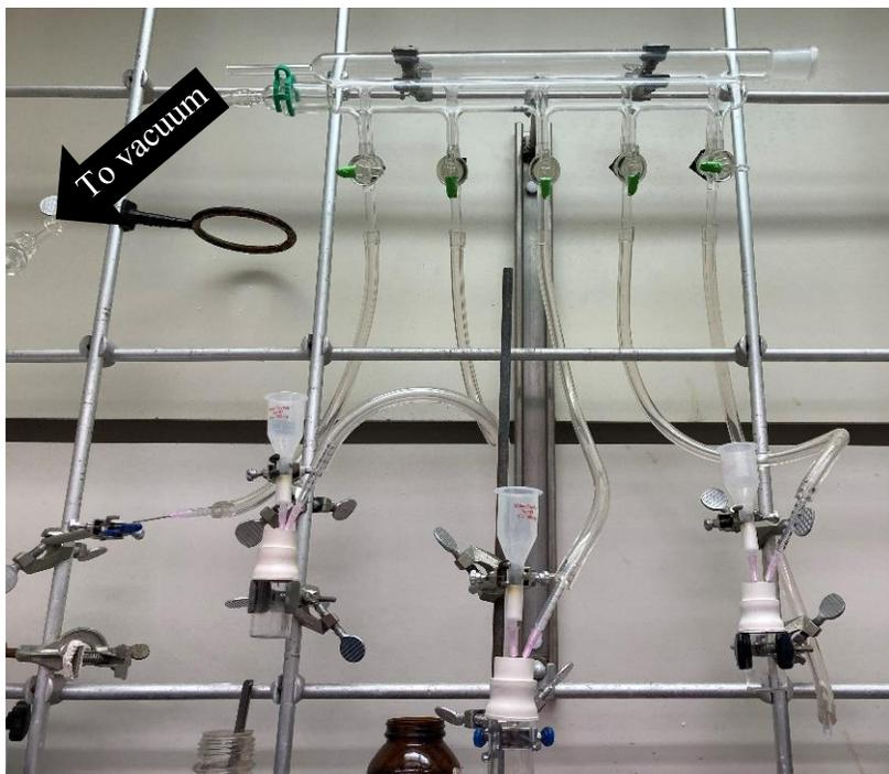
**Figure 3. Solid phase extraction (SPE) apparatus.** The vacuum was connected to the samples via a five-port vacuum gas manifold. Four samples could be run at once since the fifth stopcock was used to control vacuum pressure.
