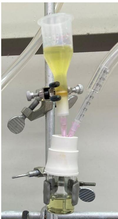
**Figure 4. SPE column apparatus.** The SPE column was connected to a syringe needle, which was inserted through a rubber septum on the collecting vial. The tube on the right connects the system to the vacuum through another syringe needle.
