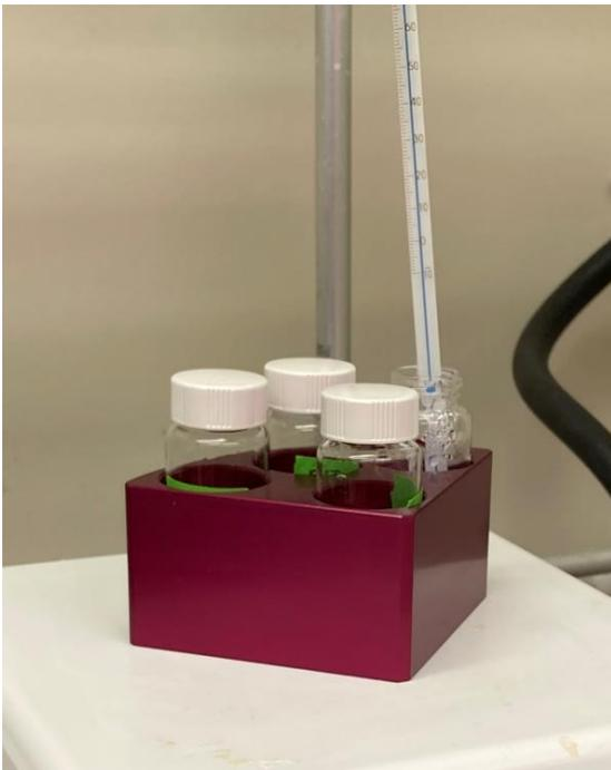
**Figure 2. Lipid extraction of ergosterol.** Samples were boiled with stirring for 30 min at 80 °C. The temperature was monitored with a thermometer in water.
