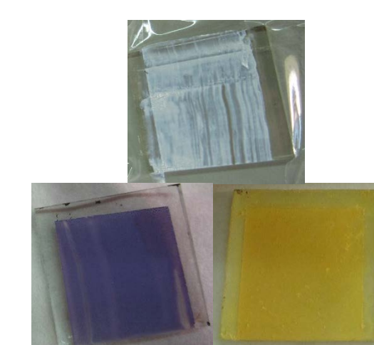
Figure 5: TiO 2 layer before and after dye absorption. Cyanidin (left), Rutin (right)
