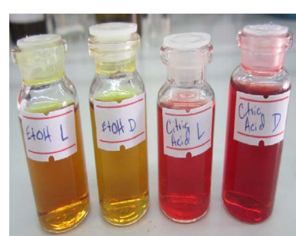
Figure 3: Ethanol and acid extracts after one week extraction
